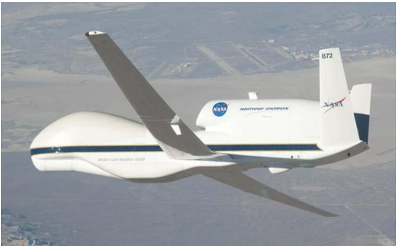
The Global Hawk can accommodate a wide range of sensors and is able to fly “untethered” from ground-based communications transmitters by using a satellite data link. The UAS navigation and communication system is comprised of a Mission Control Element and Launch and Recovery Element. These two distinct stations can be located separately and serve different functions.
